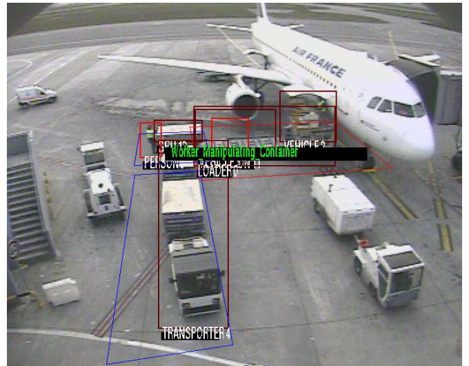
Figure 4: Two dynamic zones (in blue) linked with the Loader and the Transporter vehicles involved in the event “Worker_Manipulating_Container” (event 26) detected.
